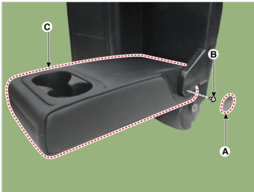
2. Remove the rear seat armrest back board (A).
